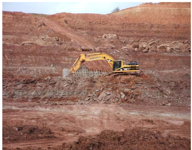
Clay being extracted from a quarry by a mechanical digger.
