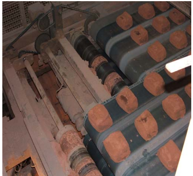
Clots of clay being mechanically thrown into moulds.
