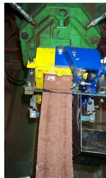
Column of extruded clay undergoing a rusticating texture
